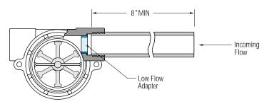
Except for straight-thread versions, RotorFlow sensors connect to piping via NPT mating thread forms. The use of an appropriate thread sealant is necessary to assure a leak-tight connection. Permatex "No More Leaks<sup>®</sup>" or 2 wraps of Teflon<sup>®</sup> tape are the only sealants recommended for GEMS flow sensors. Straight-thread versions require an O-ring for sealing.
