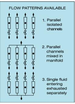
When meters with valves are ordered the valve cartridges are installed at the inlet.
