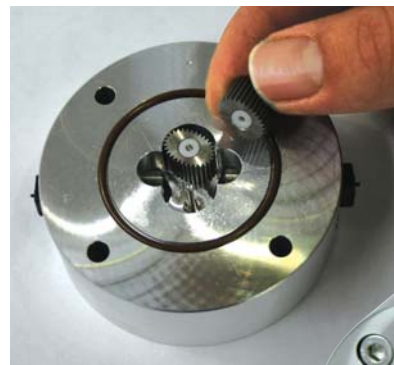
Two oval shaped gears (rotors) are the only moving parts within the measuring chamber
